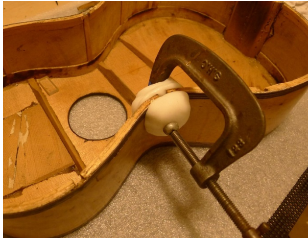
Figure 5. Correcting deformed sides. Guitar by Genaro Fabricatore, Naples 1817, New York Public Library.
