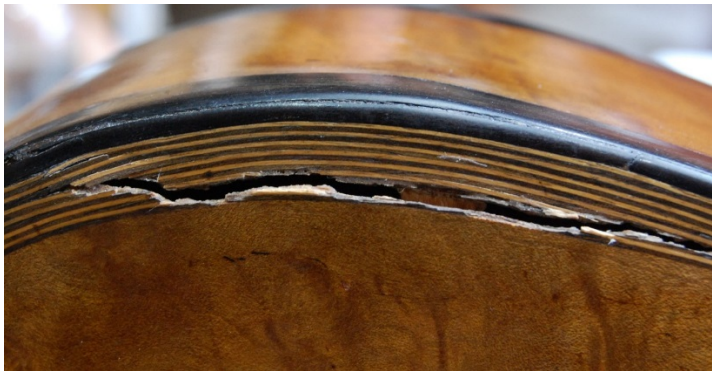
Figure 2. Fracture in the back. Guitar by Genaro Fabricatore, Naples 1825, Private collection.
