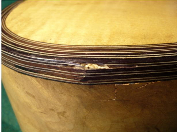
Figure 3. Fractured sides with protruding brace. Guitar by Genaro Fabricatore, Naples 1817, New York Public library.
